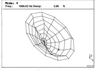
*Fig. 10. Example of an added* mass *simulation (50g at point 38). Note the downward shift in modal frequency*
