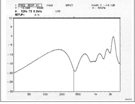
Fig. 12. A measurement showing the free field response of the driver. Structural modes contribute to the uariations in the response beyond the rigid piston range of operation
