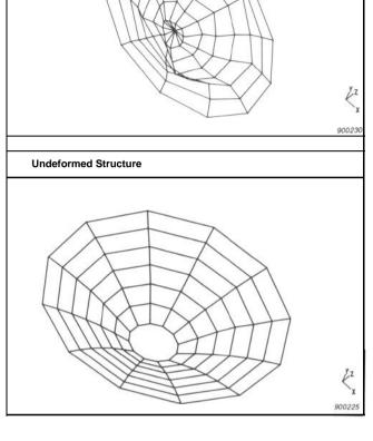
Fig. 9. Plots of the mode shapes 5, 6, 7 and the undeformed diaphragm.
