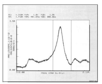
Fig. 7. An example of a curve-fit to a particular mode in a single FRF
