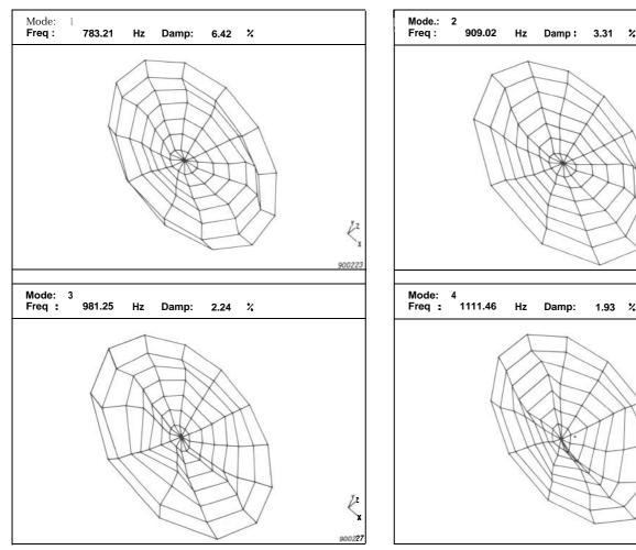
Fig. 8. Plots of the mode shapes 1, 2, 3, and 4. For each mode shape, the modal frequency and damping are listed above the structure
