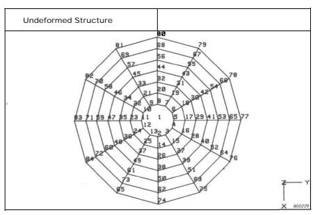
Fig. 5. Measurements were performed at 73 diff erent points around the diaphragm. No measurements were made at the points numbered from 74 to 85. These points represent the driver frame and are used as a reference for the displacement
