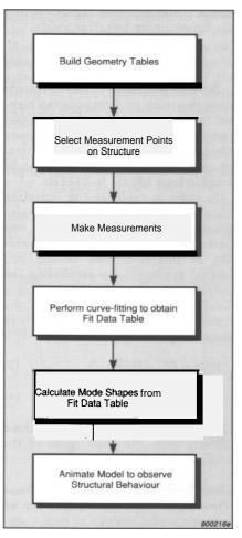
Fig. 2. Procedure for a general modal test
